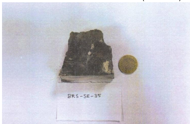
Figure 13. Sample number BRS-SE-35. The rock appears fine grained dark grey in colour with stringers.
