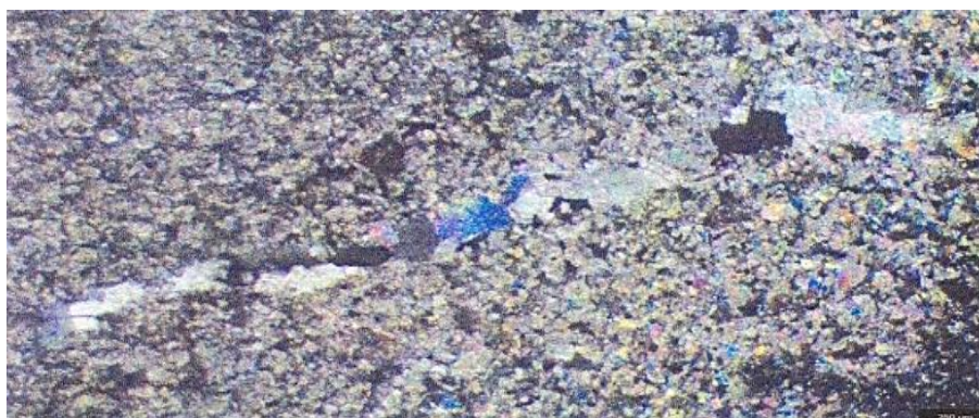
Figure 17. Sample number BRS-SE-41. Photomicrograph illustrates a calcite-quartz rich veins traversing through a medium-fine grained carbonate rich micritic matrix, predominantly composed of calcite. Under XPL (2.5X).
