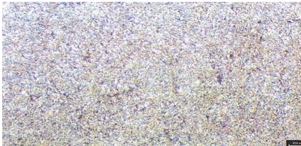
Figure 9. Photomicrograph of BRS-SE-25. Photomicrograph reveals fine grained microcrystalline carbonates embedded in micritic matrix. Under XPL.
