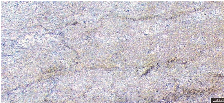
Figure 7. Photomicrograph of sample number BRS-SE-22. Photomicrograph reveals very fine-grained microcrystalline carbonates embedded in muddy matrix. Under XPL (2.5X).
